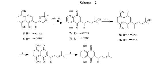
Reagents and conditions: a) TBAF, THF, rt, 3 h, 87%; b) Ac<sub>2</sub>O, pyridine, 0°C, 2 h, 89%; c) pyridine, SOCl<sub>2</sub>, -20°C, 27%; d) 1 mol/L NaOH, then 2 mol/L HCl, 31%.
